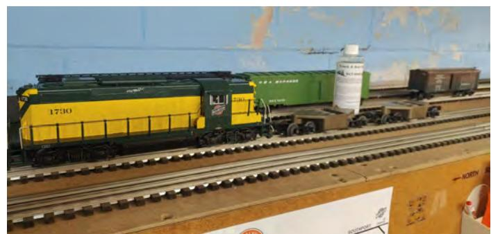
nuts and bolts inside for weight to help them roll down the track. The lead car roller has been slightly moistened with the solution and the second one is dry to help collect the moisture off the track. I find this solution doesn't leave a film on my track and cause problems with operation. If more serious cleaning needs to be done I like to use the fine side of a 3M abrasive sponge or a Walthers Bright Boy.
