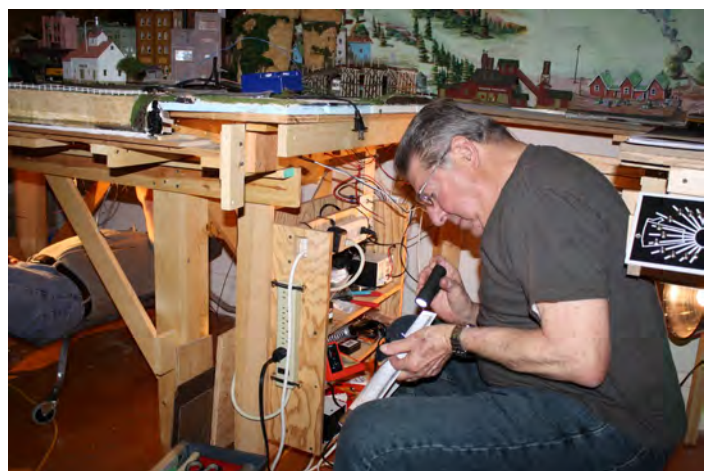
The pictures above and to the left show Nate soldering in feeder wires for roundhouse lighting, adding sub roadbed for a mainline realignment, installing relays and power supplies for our conversion to DCC, and acting as switchman during an operating session, along with engineer Larry Wierer.
