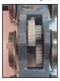
drive axle meshed with the reduction gear and the motor removed making sure the gears do not bind. I have seen these molded gears far enough out of true that they bind. Sometimes you can rotate the driver to a different mesh position of the reduction gear and fix this. Then you
