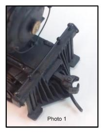
This metal coupler clears most pilots and requires the frame of the locomotive to be electrically isolated. It is for this reason that I always use drivers that completely insulate the frame from the rails. You may notice that one of the driver centers
