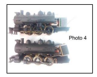
There are many modern smaller motors that can be used which have better performance, lower stall current and are more decoder friendly. This locomotive is small so most any size motor 12mm or so will be fine. A flat can motor is good choice and there is a seller on eBay, cvbackshop, that makes a conversion kit for this locomotive. A motor from MDC 2-6-0 or 2-8-0 "old timer" with the reduction gear will do the job and already has the correct worm gear fitted to the motor, Photo 5.
