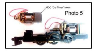
If you chose to adapt your own motor, you will likely need a sleeve to match the worm gear hole to your motor shaft diameter. I routinely make these sleeves on my lathe. NWSL makes these sleeves in various sizes, also.
